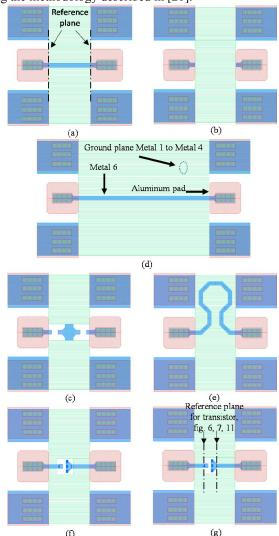
Fig. 2: Simplified representation of the layout of some of the test structures (through, reflect, line, transistor open, meander line, transistor): (green horizontal line) is M1 to metal 4 (Ground plane), blue dotted is metal 6, red right-hatched is aluminum used for the pad. The probe pitch is 50  $\mu m.$  a) Thru of  $50\mu m,$  b) Reflect, c) Line of  $160\mu m,$  d) Load, e) Meander line, f) Transistor open, g) Transistor.
