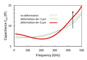
Fig. 15: Capacitance "C22" versus frequency of the transistor-open obtained from EM simulation including a TRL calibration with an ideal probe and with defaults  $(dx=3\mu m, sx=6\mu m)$  when simulating the transistor open.
