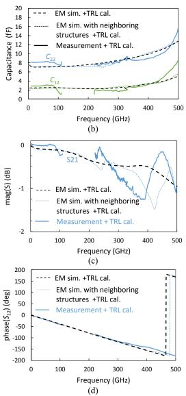
Fig. 5: S parameter measurements with on-wafer TRL calibration and comparison to several EM simulations for: a) magnitude of S parameters and b) capacitance of a transistor-open, c) magnitude and d) phase of a meander line up to 500 GHz.
