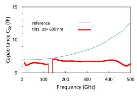
Fig. 9: Capacitance " $C_{22}$ " versus frequency of the transistor-open obtained from EM simulation including a TRL calibration with an ideal probe and with tilt default (reference:  $\Delta z$ =0nm, tilt1:  $\Delta z$ =600nm).
