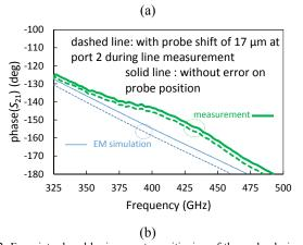
Fig. 12: Error introduced by inaccurate positioning of the probe during Line standard measurement when performing TRL calibration with ZC (characteristic impedance of the line) correction: impact on a) the capacitance of the transistor-open and b) the phase of the meander line. (solid line: TRL set 1 with contact 1, dotted line: TRL set 2 with contact 2)
