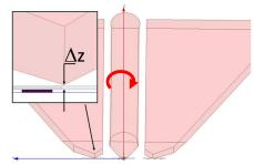
Fig. 8: EM model used for planarity of the probe (reference:  $\Delta z$ =0nm, tilt1:  $\Delta z$ =600nm contact is lost in the last case)
