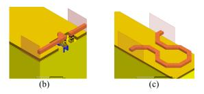
Fig. 3: Geometrical model for EM simulation including neighboring structures of a) the EM full structure including probes, pad open and b) half intrinsic transistor open c) intrinsic meander line (wave ports correspond to reference plane of the TRL calibration). (gold: metal 1 bis metal 5, orange: metal 6, yellow: Si, brown SiO2).
