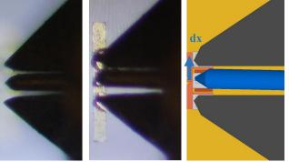
Fig. 14. Image of a 50 µm pitch CPW probe a) before contact and b) after contact on a used ISS short standard. The probe flexibility in combination with a deteriorated ISS standard causes a deformation of the probe eventually modifying its characteristic impedance; c) Geometrical Model for EM simulation showing a default on CPW probe (dx=6µm movement at port 2).
