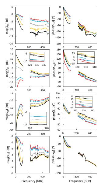
Fig. 7: S parameter measurements of a 2\*CBEBC SiGe HBT of  $(0.22*1\mu m^2)$  drawn emitter size from Infineon for different  $V_{BE}$  ranging from 0.7-0.94 V with 60 mV step and  $V_{CB}$ =0 V, using an on-wafer TRL calibration with impedance correction and move of the reference plane above vias at M6 (see Fig. 2); magnitude and phase.
