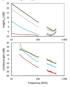
Fig. 6: Unilateral gain and Current gain H21 of a 2\*CBEBC SiGe HBT of  $(0.22*1\mu\text{m}^2)$  drawn emitter window size from Infineon for different  $V_{BE}$  ranging from 0.7-0.94 V with 60 mV step and  $V_{CB}$ =0 V, using an on-wafer TRL calibration with impedance correction, plus move of the reference plane above vias at M6 (see Fig. 2).
