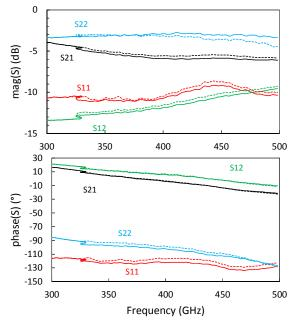
Fig. 13: Error introduced by inaccurate positioning of the probe during Line standard measurement when performing TRL calibration. Transistor measurement at  $V_{BE}$ =0.9V and  $V_{BC}$ =0V - TRL calibrated and ZC (characteristic impedance of the line) corrected S parameter measurement and same reference plane as Fig. 6 . (solid line: TRL set 1 with line contact 1, dotted line: TRL set 2 with line contact 2)
