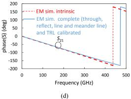
Fig. 4: Comparison of EM simulation of the on-wafer TRL calibration (blue) with EM simulation of the intrinsic device (red-dashed) for a) magnitude of S-parameter and b) capacitance for the transistor-open and c) magnitude of S-parameter and d) phase for the meander line.
