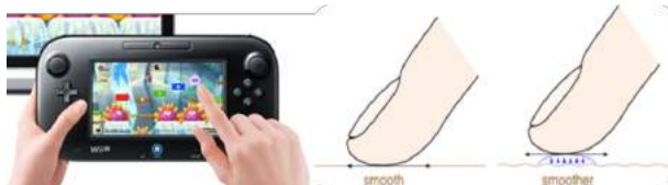
Figure 11: Haptic screen, the modulation of stationary waves gives different feeling when touching the surface
