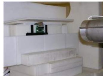
Figure 2: The DUT facing the neutron source
