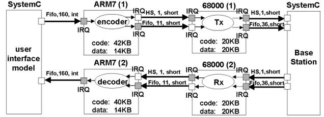
Figure 5. A macro-architecture specification of IS-95 system.
