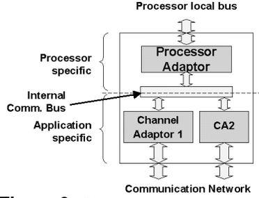
Figure 3. Communication coprocessor.
