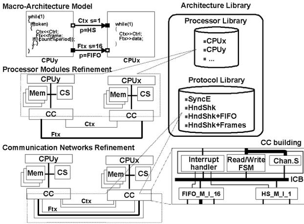
**Figure 7.** Architecture generation flow.
